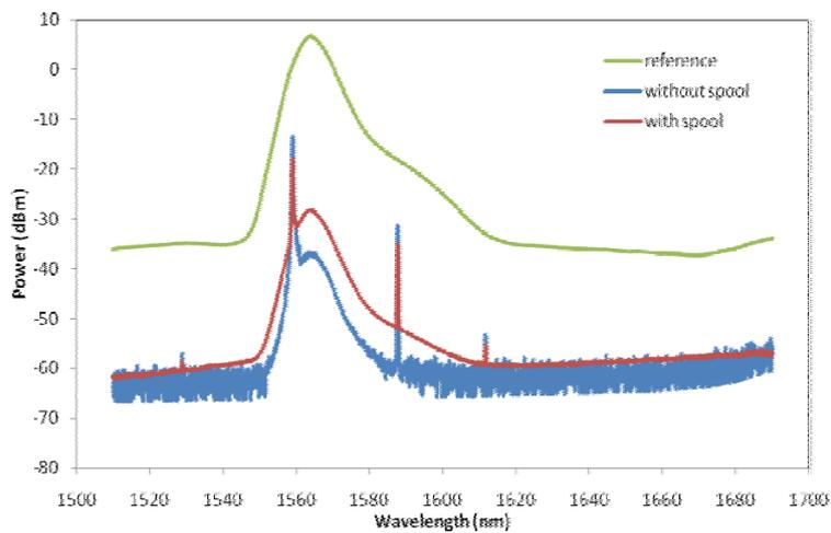
Figure 11. Spectral power measurements obtained for the setup of Fig. 2 employing the ASE power of the EDFA-L amplified by the EDFA-C (resolution of 0.06 nm).
