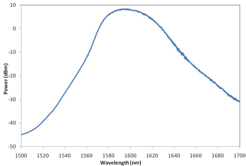
Figure 4. Spectral power emitted by the mode-locked laser with the EDFA-C as active medium and the EDFA-L as post-amplifier. The OSA resolution is 1 nm.
