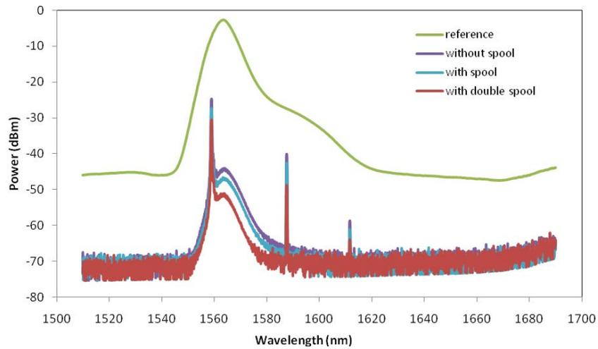
Figure 7. Spectral power measurements obtained for the setup of Fig. 1 employing the ASE power of the EDFA-C amplified by the EDFA-L (resolution of 0.06 nm).
