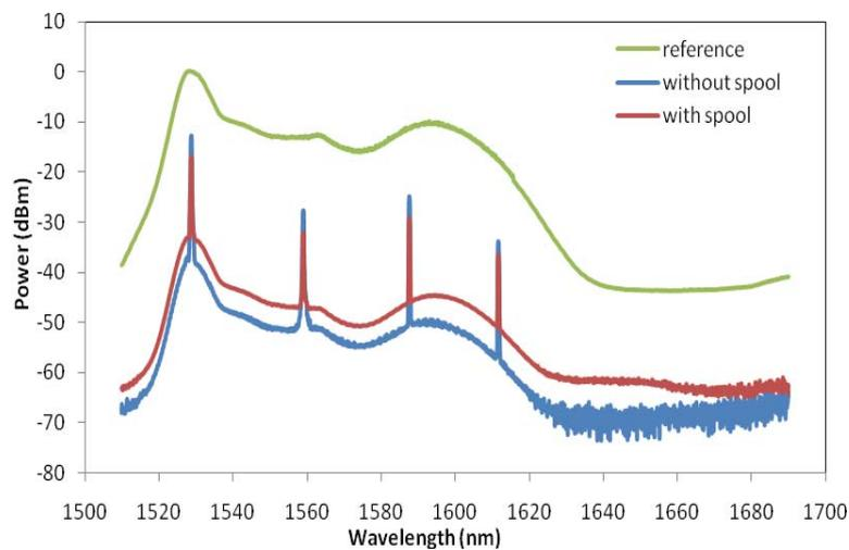
Figure 13. Spectral power measurements obtained for the setup of Fig. 2 employing mode-locked pulses amplified by the EDFA-C (resolution of 0.06 nm).
