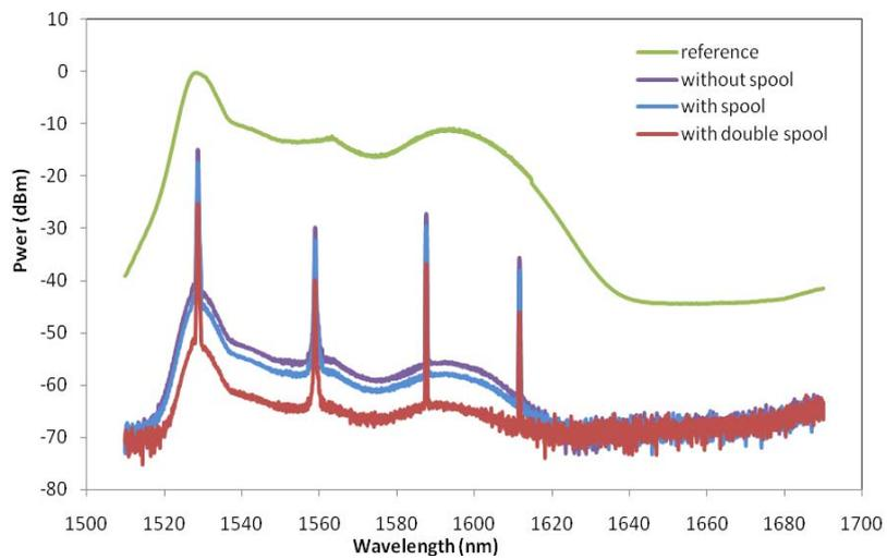
Figure 9. Spectral power measurements obtained for the setup of Fig. 1 employing mode-locked pulses amplified by the EDFA-C (resolution of 0.06 nm).
