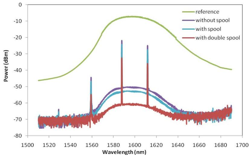
Figure 8. Spectral power measurements obtained for the setup of Fig. 1 employing mode-locked pulses amplified by the EDFA-L (resolution of 0.06 nm).
