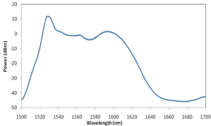
Figure 5. Spectral power emitted by the mode-locked laser with the EDFA-L as active medium and the EDFA-C as post-amplifier. The OSA resolution is 1 nm.
