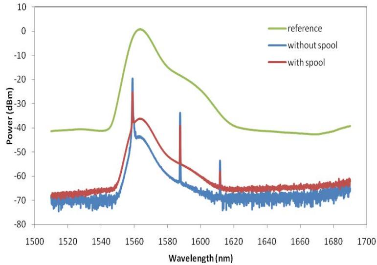
Figure 10. Spectral power measurements obtained for the setup of Fig. 2 employing the ASE power of the EDFA-L (resolution of 0.06 nm).
