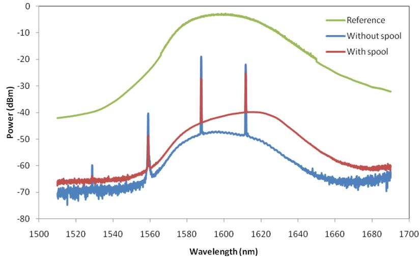
Figure 12. Spectral power measurements obtained for the setup of Fig. 2 employing mode-locked pulses amplified by the EDFA-L (resolution of 0.06 nm).
