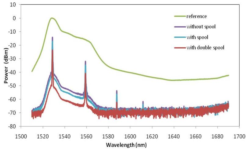
Figure 6. Spectral power measurements obtained for the setup of Fig. 1 employing the ASE power of the EDFA-C (resolution of 0.06 nm).
