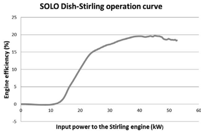
Fig.2 SOLO dish-Stirling operation curve (Reinalter, 2005)
