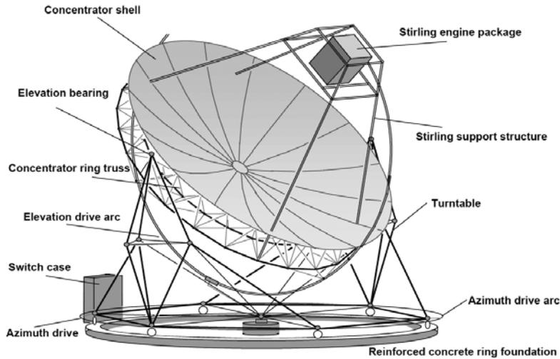
Fig.1 Dish-Stirling thermosolar generation system sketch (Schiel, 2001)
